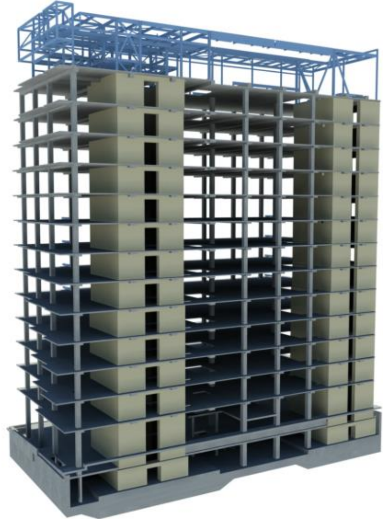
Concrete with PT cores
