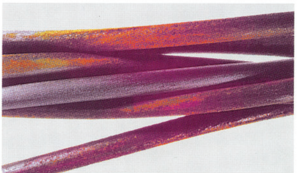
Photo 8A. Strand surface after cleaning
