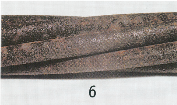
Photo 6. Strand surface before cleaning
