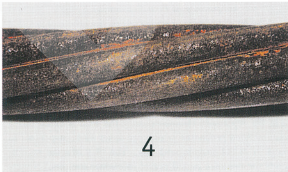
Photo 4. Strand surface before cleaning
