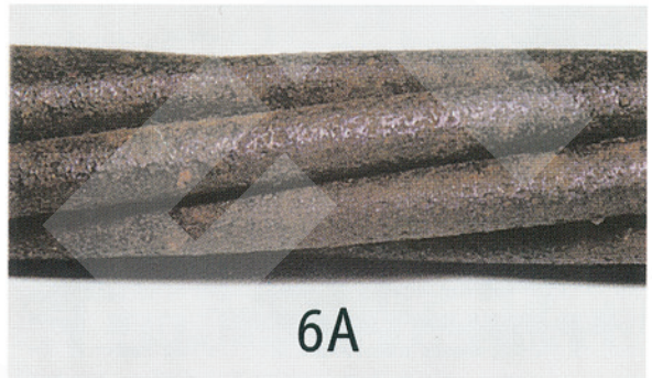
Photo 6A. Strand surface after cleaning
