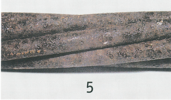
Photo 5. Strand surface before cleaning
